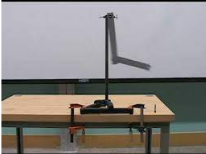
Figure 6. A double pendulum constructed from similar uniform slabs; a frame from a demonstration video by YouTube user stevenbtroy [11].
