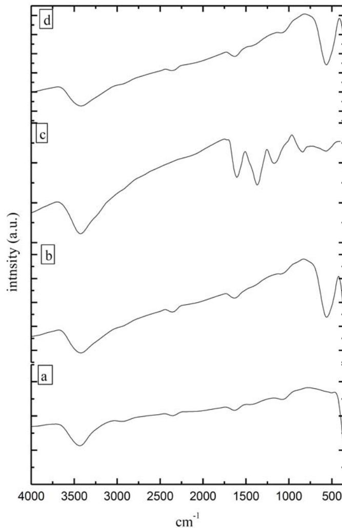
**Figure 4.** FTIR spectrum of (a) pr-G, (b)  $\text{MnO}_x$ -G composite, (c) MB dye, and (d)  $\text{MnO}_x$ -G composite after interaction with the dye solution.
