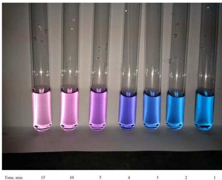
**Figure 10.** Change in the color of dye with the treated time of  $\text{MnO}_x\text{-G}$  ( $[\text{MB}] = 100\text{ppm}$ , catalyst dose =  $0.2\text{g}/20\text{ml}$ ,  $T = 25^\circ\text{C}$  and  $\text{pH} = 1.5$  for 0-15 min).
