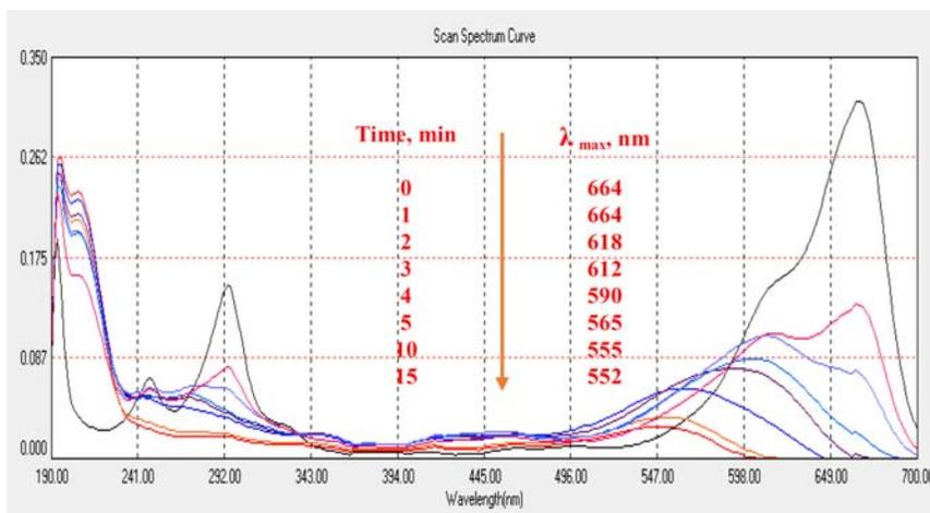
**Figure 9.** The UV-Vis spectra in the range of 190-700nm of MB-dye ([MB] = 100ppm, catalyst dose = 0.2g/20ml, T = 25°C and pH = 1.5 for 0-15 min).
