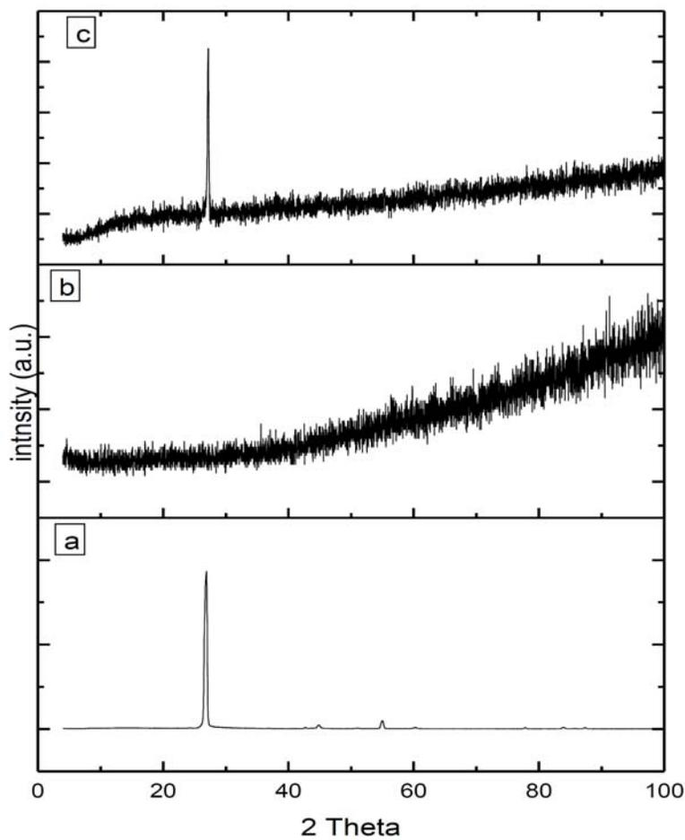
**Figure 2.** XRD patterns of (a) pr-G, (b)  $\text{MnO}_x$ , and (c)  $\text{MnO}_x$ -G composite.
