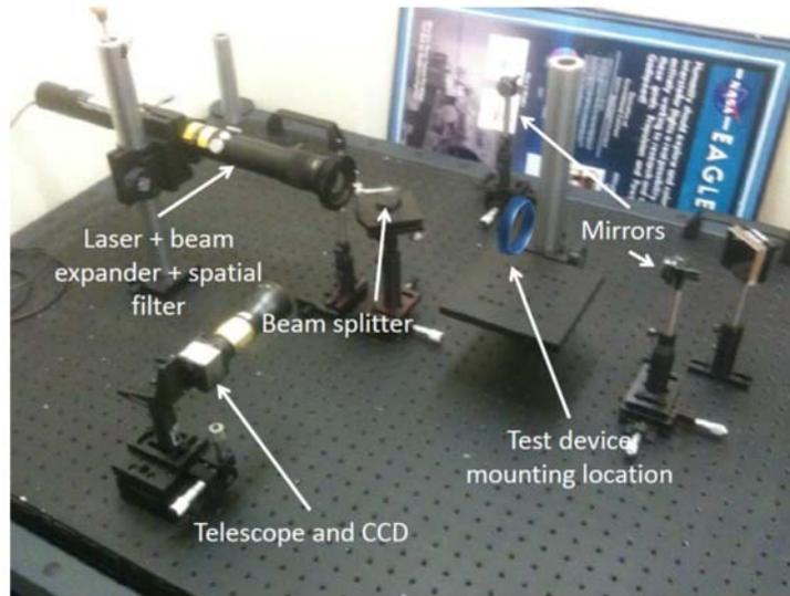
**Figure 1.** The White-Juday Warp Field Interferometer<sup>1</sup>.
