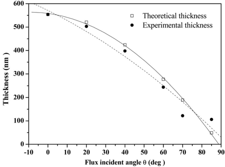
**Figure 6.** Thickness of  $\text{CuInS}_2$  thin films varies with the incident flux angle.
