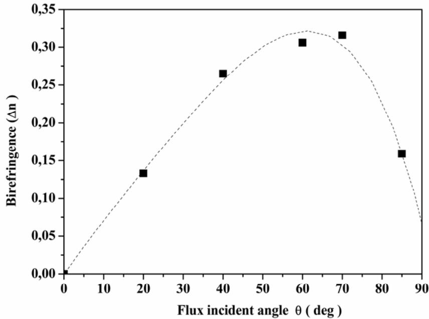
**Figure 10.** In-plane birefringence  $\Delta n$  ( $\lambda = 1350\text{nm}$ ) of CuInS<sub>2</sub> thin films.
