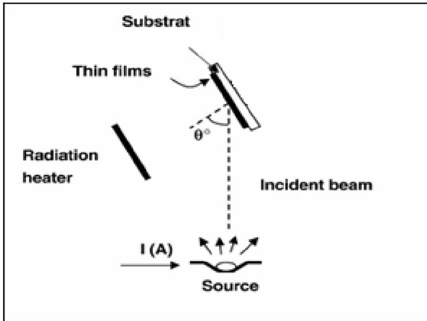
**Figure 1.** The schematic diagram of the GLAD technique.
