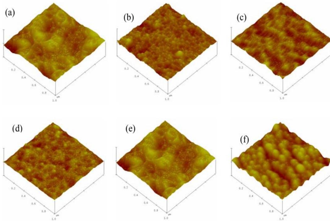
**Figure 4.** AFM images of  $\text{CuInS}_2$  films deposited at different incident angles.
