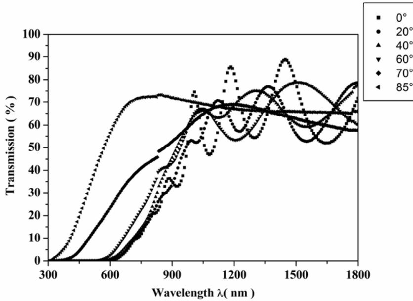
**Figure 7.** Transmittance spectra of  $\text{CuInS}_2$  thin films deposited at different incident angles.
