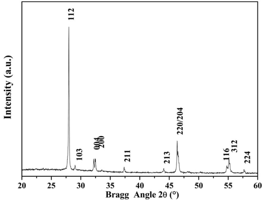
**Figure 2.** XRD patterns of  $\text{CuInS}_2$  powder.
