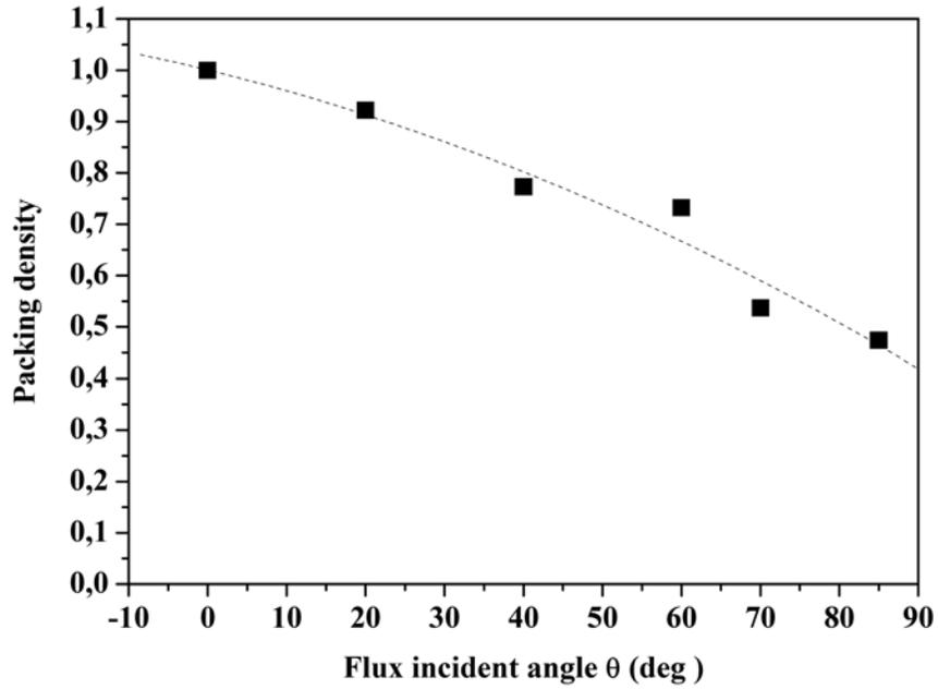
**Figure 9.** Packing density ( $\lambda = 1350\text{nm}$ ) of CuInS<sub>2</sub> thin films at different deposition angle.
