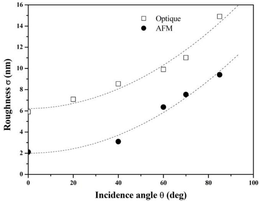
**Figure 5.** Optical and AFM measurements of surface roughness parameter of  $\text{CuInS}_2$  thin films.
