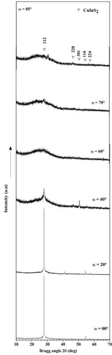
**Figure 3.** XRD patterns of CuInS<sub>2</sub> thin film deposited at different incident angles.
