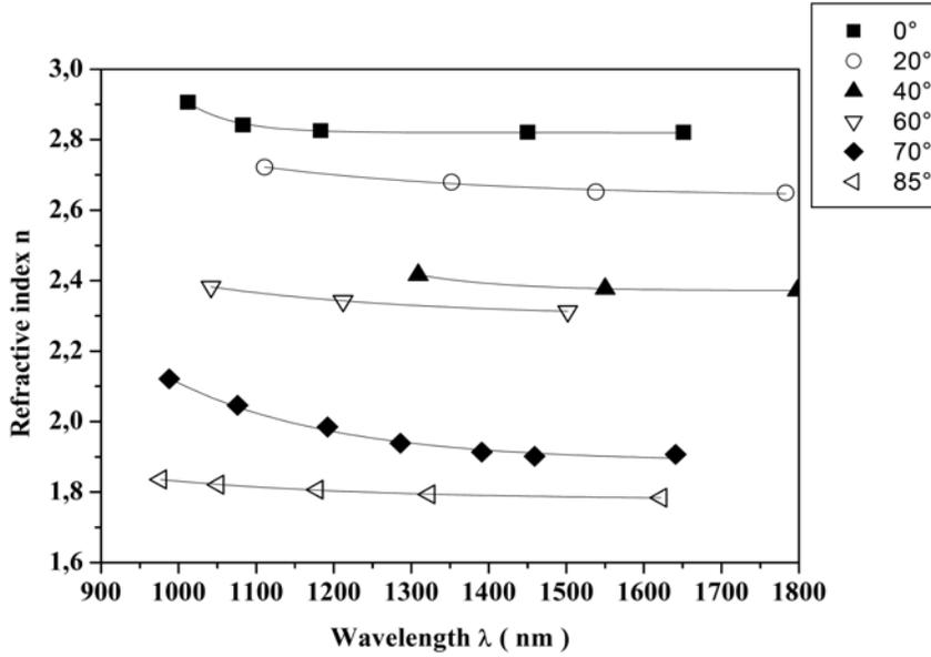
**Figure 8.** Refractive indices of  $\text{CuInS}_2$  thin films deposited at different incident angles.
