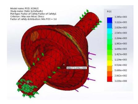
**Figure 9.** The distribution of the safety factor for the destruction of steel with a minimum value of FOS = 3, 63.
