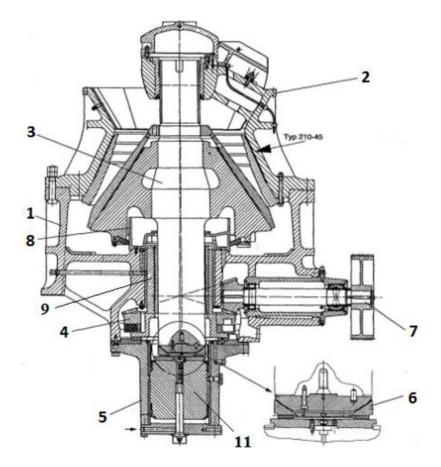
Figure 1. Conical crusher for medium crushing with two-sided movable cone type "KUBRIA" 210/35 [2].
