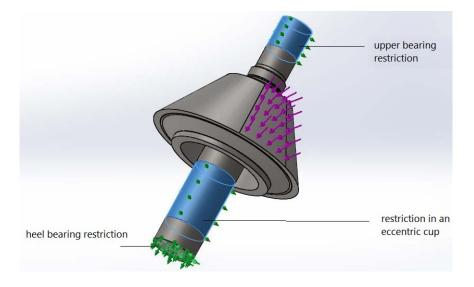
Figure 4. Fixed surfaces and constraints of the movable cone and the crusher shaft.
