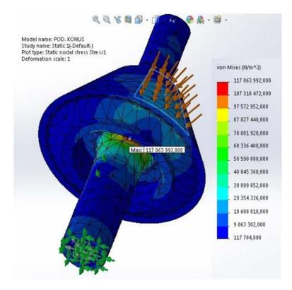
Figure 7. Zone of maximum stress at the component.
