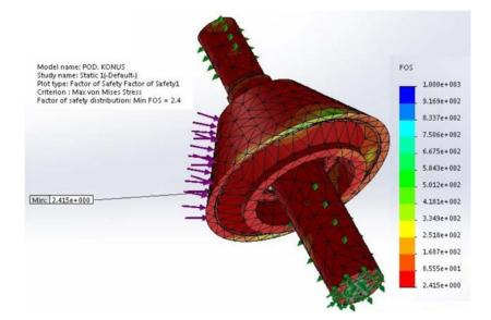
**Figure 8.** The distribution of the steel safety factor for pulling with a minimum value of FOS = 2, 42.
