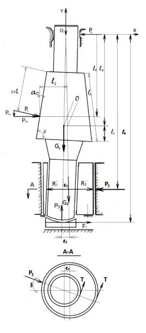
Figure 2. Kinematic scheme of the crusher "KUBRIA" 210/35 [2].
