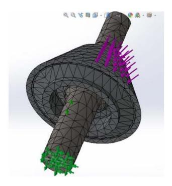
Figure 5. Discretization of the model with the applied crushing force.
