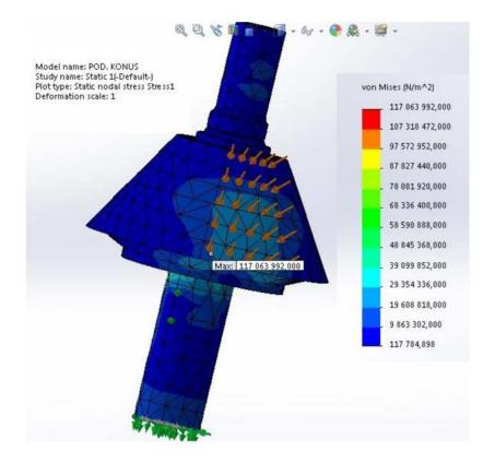
Figure 6. Distribution of the equivalent stress in a node movable coneshaft at a 6081kN.
